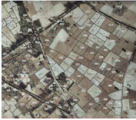
Vectorised field map showing the resulting cadastral map with parcel boundaries and cadastral numbers.
